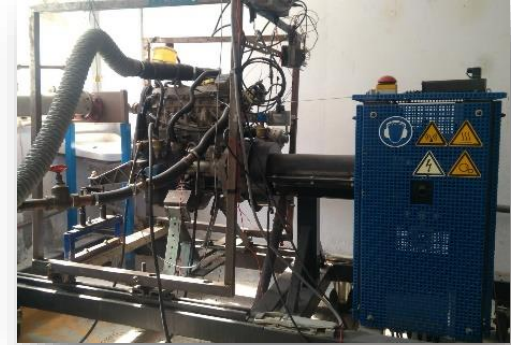
Motor Manyetik Fren Test Cihazı (Computest)
